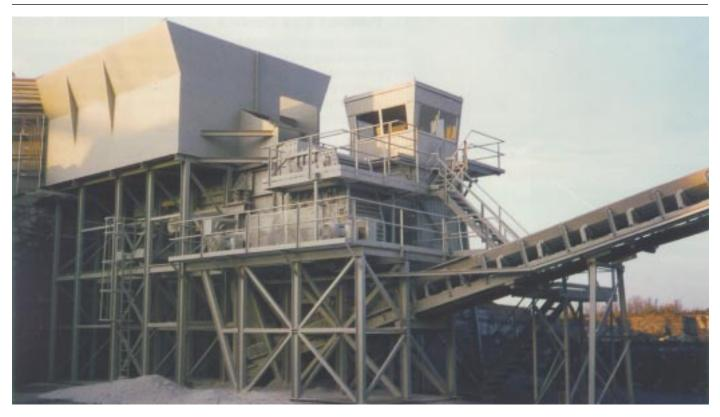
Single impeller impact breakers can be skid-mounted or portable. Skid units, which can include feeder, grizzly and drive, are completely engineered and ready to install on piers. Portable units have the same components and a discharge conveyor on a single chassis for easy transport. Electric motor or combustion engine provide power.
